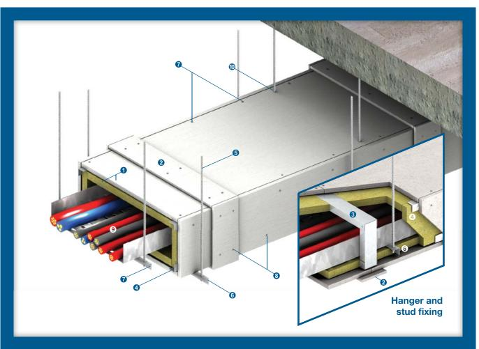
Up to 120/120/120 or 240/240/240 fire resistance in accordance with the requirements of BS 476: Part 20: 1987 and AS 1530: Part 4: 2005
