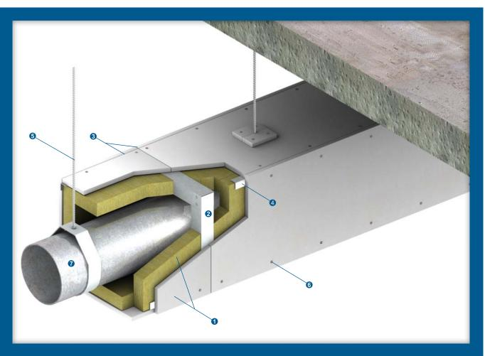
Up to 120/120/120 or 240/240/240 fire resistance in accordance with the requirements of BS 476: Part 20: 1987 and FSB/PSB/001/00 test procedure
