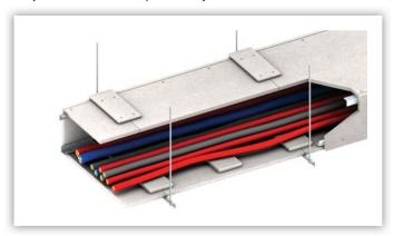
The enclosure system must be supported, either by direct fixing to other structural elements with suitable proprietary steel fixings or by hangers at maximum centres of 1220mm. The hanger supports should coincide with enclosure joints. The hangers consist of steel threaded rods and a steel angle bearer section under the protection system. The tensile and bending stresses of the unprotected hangers and bearers must not exceed 10N/mm² for up to 120 minutes fire resistance.
