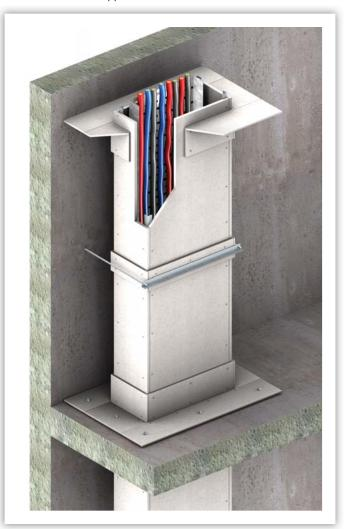
The weight of the enclosure assembly must be fully supported at each floor level. Steel angles may be fitted to the enclosure at floor penetration level and sit upon the floor slab, supporting the weight of the enclosure.
