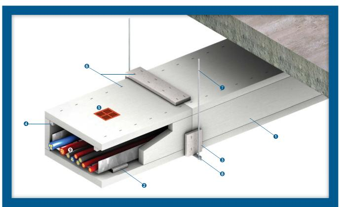
Up to 120/120/120 fire resistance in accordance with the requirements of BS 476: Part 20: 1987 and AS 1530: Part 4: 2005
