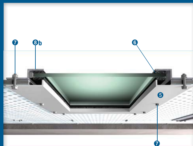
Fixing details of vision glass
