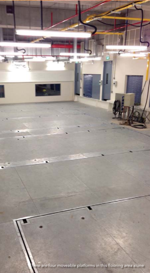
Moveable platform with up to 20kN/mm 2 of loading capacity
