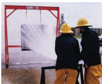
ABOVE: DURASTEEL® undergoing 3.1Bar high pressure hose stream test, in accordance with ASTM E119 requirements.
