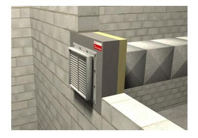
Dampers and ducts should penetrate separating walls in their own aperture be sealed in line with the service manufacturers tested systems.
