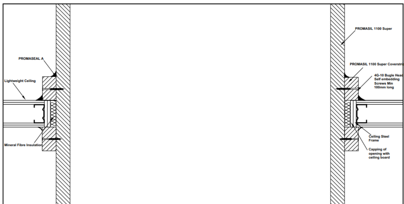
Figure 20 Vertically oriented duct through fire rated lightweight floor and/or ceiling system
