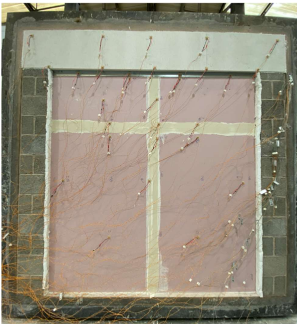
Fig 1.1 – Testing rig set up with thermocouples in place prior to placement into fire testing furnace.
