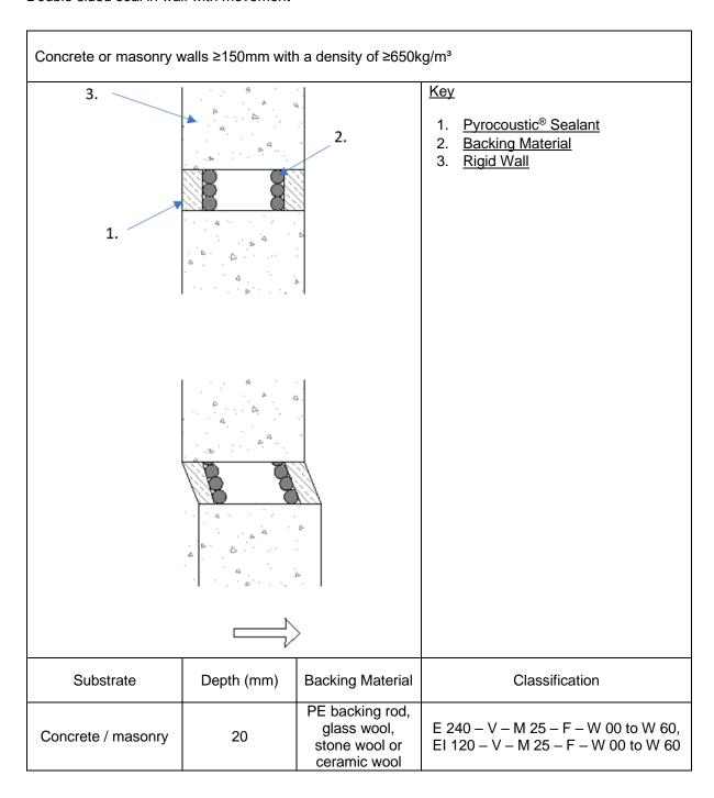
Single sided linear joint in wall with movement
