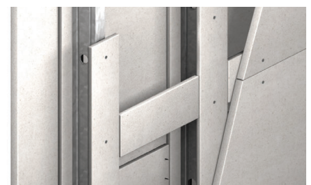
Horizontal joints with board strips
