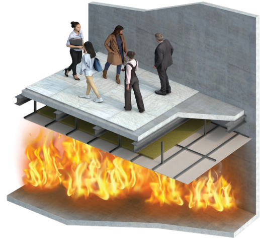
Protection to structural loading bearing floor
