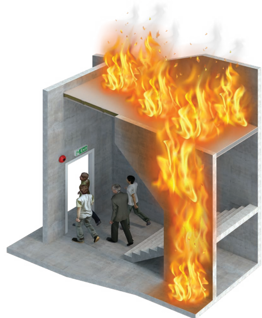
Protection for escape route - staircase
