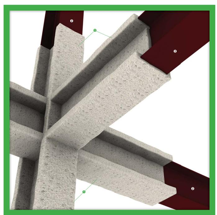
Up to 240/-/- fire resistance in accordance with the requirements of BS 476: Part 21: 1987 and/or UL 1709
