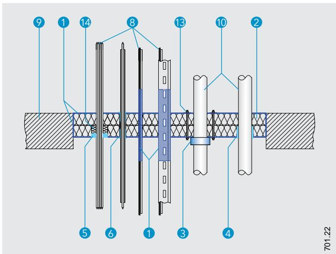
**Detail B - Mixed penetration seal in rigid floor**
