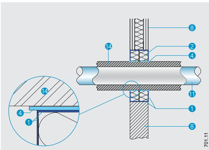
**Detail Y - MLC pipe penetration seal in flexible and rigid wall**
