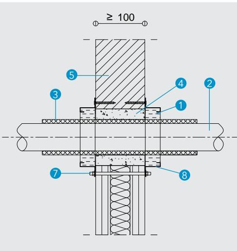
**Detail W** - Mortar penetration seal of metal pipes with combustible insulation, sealed with use of PROMASTOP®-FC MD in flexible or rigid wall
