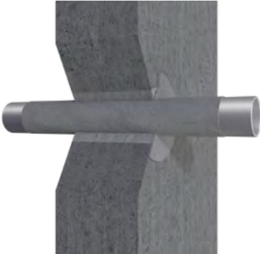
In case of supporting constructions with timber studs no part of the penetration seal is closer than 100 mm to a stud, the cavity is closed between the penetration seal and the stud and minimum 100 mm of insulation of class A1 or A2 according to EN 13501-1 is provided within the cavity between the penetration seal and the stud.
