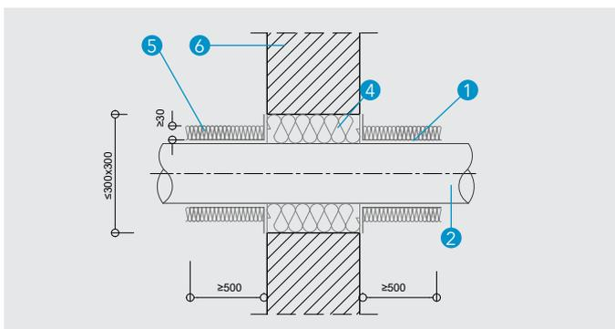
**Detail C - Penetrations of steel or cast iron pipes up to 114 mm through rigid walls**
