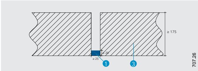
**Detail P - Joint seal on the bottom side of the floor without backfilling**
