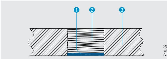
**Detail F - Joint filling coated on the exposed side in floor**
