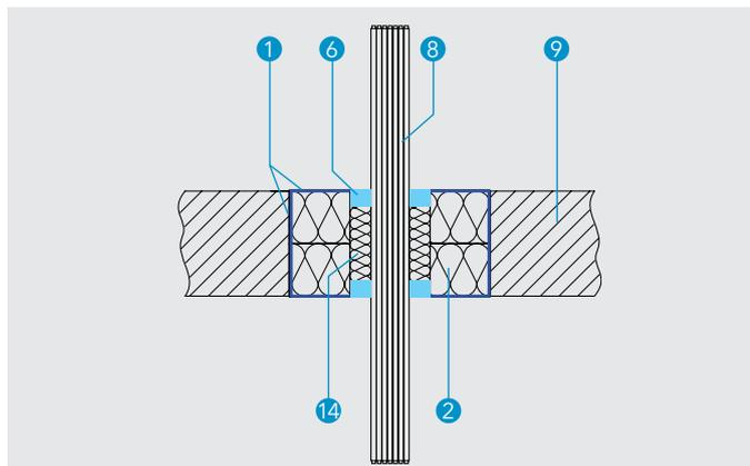
**Detail U - Cable penetration seal in rigid floor**
