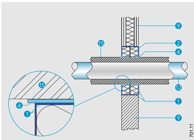
**Detail AD - MLC pipe penetration seal in flexible and rigid wall**
