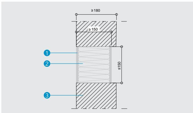
**Detail B - Double-sided protection of expansion joints**
