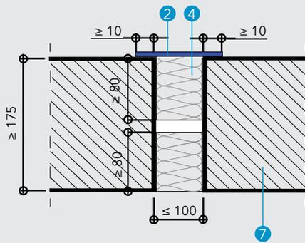
**Detail C - Joint filling coated on the unexposed side in floor**
