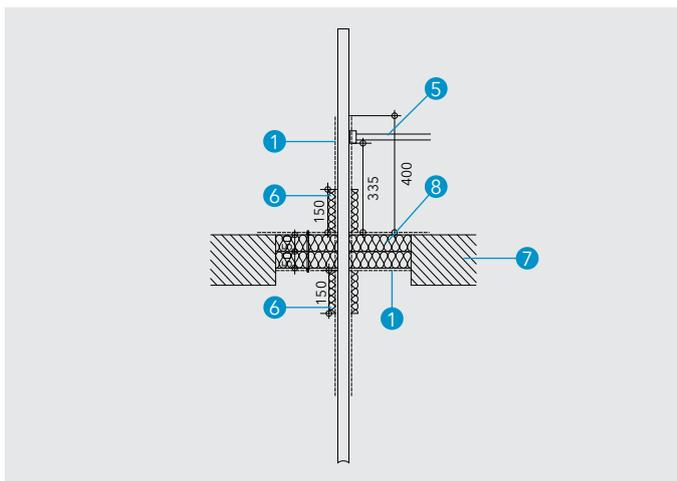
**Detail G - Soft penetration seal of metal pipes with mineral wool insulation in rigid floor, sealed with use of PROMASTOP®-A spray**
