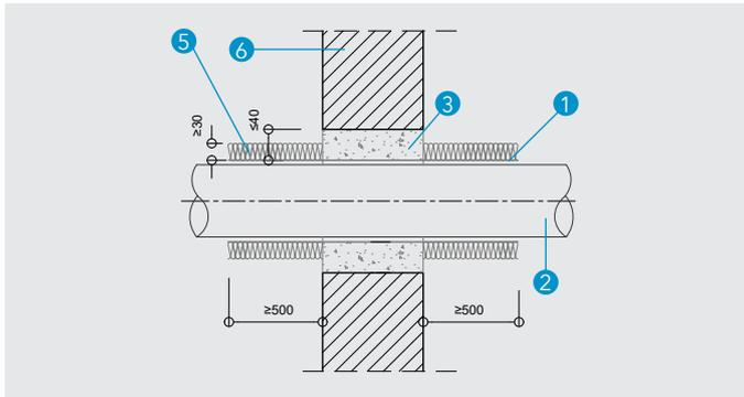
**Detail A - Penetrations of steel or cast iron pipes diameter exceeding 42 mm through rigid walls**
