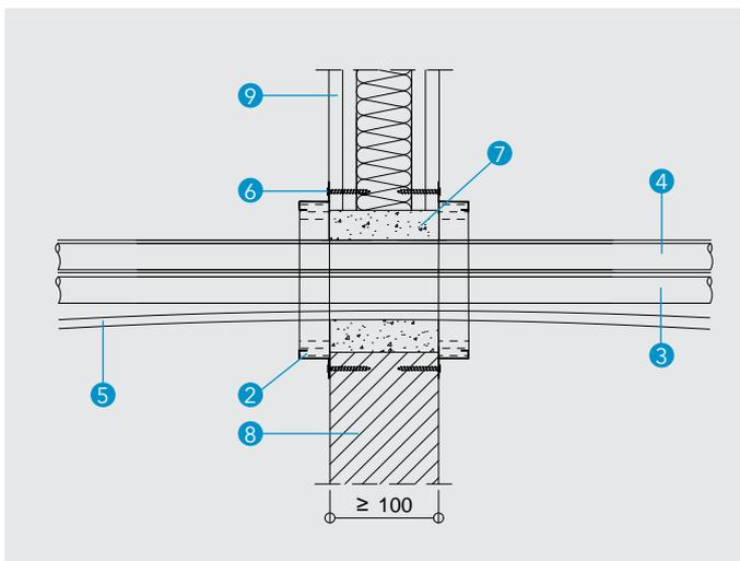
**Detail T - Mortar penetration seal of mixed bundles, sealed with use of single PROMASTOP®-FC MD in flexible or rigid wall**
