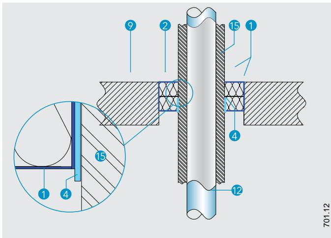
**Detail AC - MLC pipe penetration seal in rigid floor**
