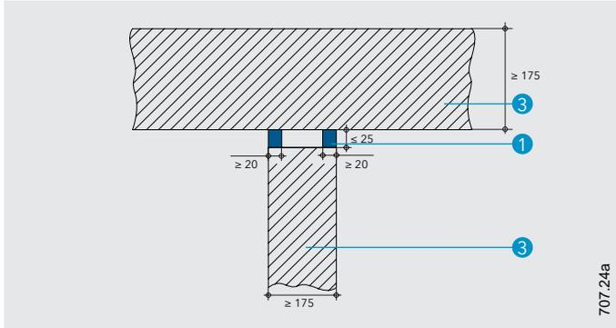
**Detail K - Joint seal without backfilling in wall (floor connection)**
