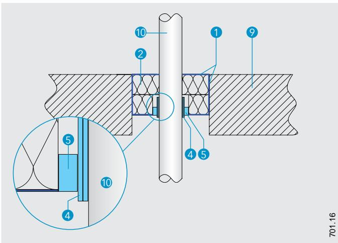
**Detail Z - Plastic pipe penetration seal in rigid floor**
