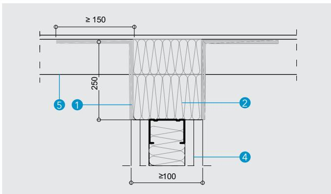
**Detail B - Protection of expansion joints between flexible walls and rigid floors**
