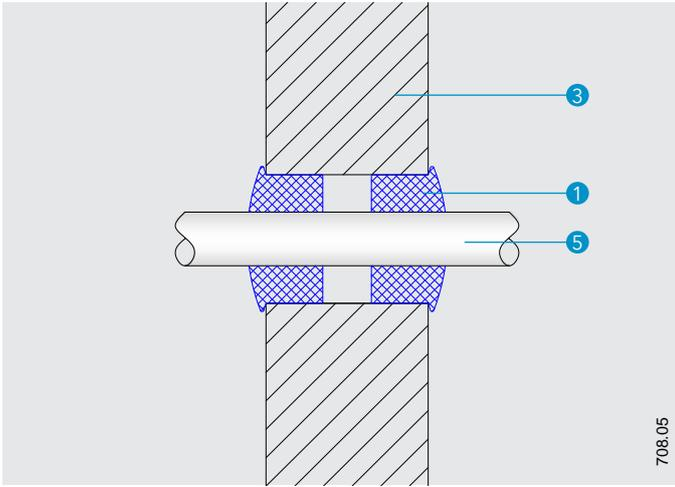
**Detail D - PROMASTOP®-P plastic pipe penetration seal in rigid wall**
