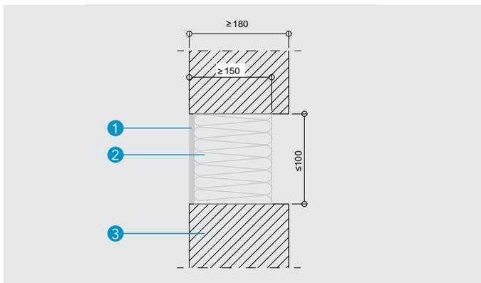
**Detail A - One-sided protection of expansion joints**
