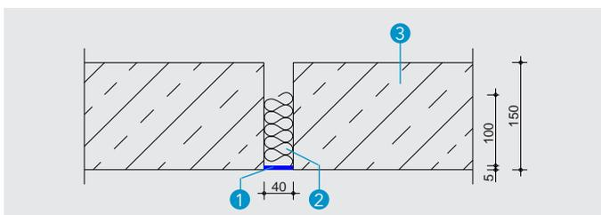
**Detail R** - Mineral wool backfilling coated on the exposed side in floor
