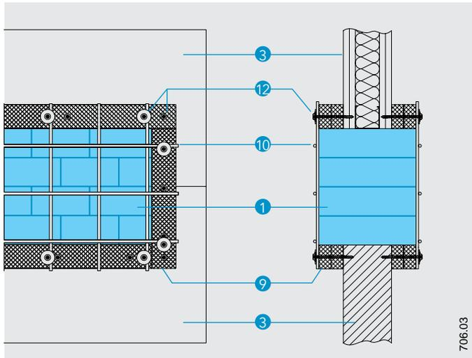
**Detail C - PROMASTOP®-B blank seal in flexible and rigid wall**
