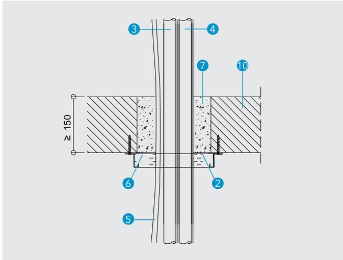
**Detail U - Mortar penetration seal of mixed bundles, sealed with use of single PROMASTOP®-FC MD in rigid floor**
