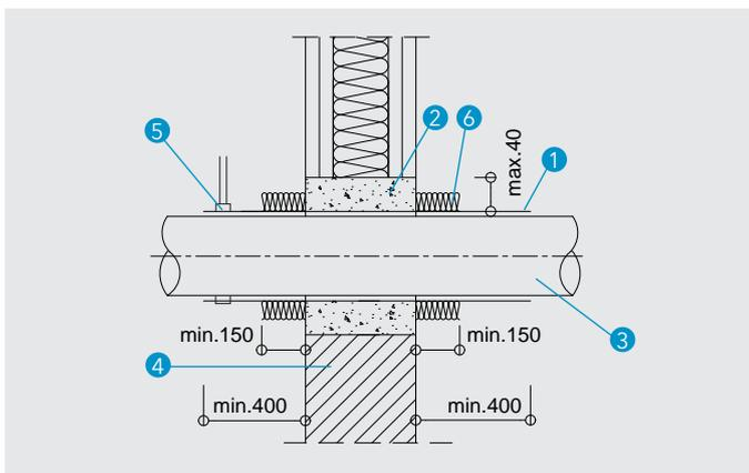
**Detail D - Mortar penetration seal of metal pipes with mineral wool insulation in flexible or rigid wall, sealed with use of PROMASEAL®-A spray; the length of the pipe insulation is less than the length of the coating on the pipe**
