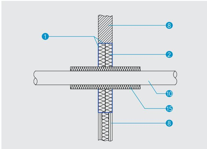
**Detail I - Metal pipe penetration seal in flexible and rigid wall in LS configuration**
