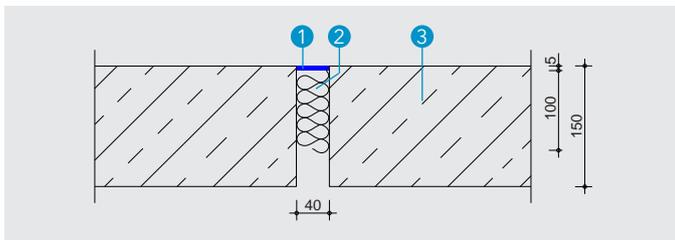
**Detail Q** - Mineral wool backfilling coated on the unexposed side in floor
