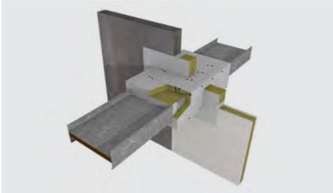
**Detail AG - Lining of a busbar system**
