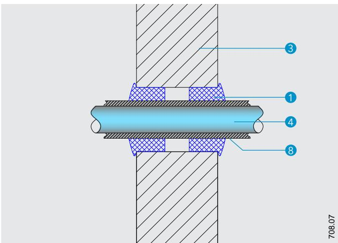
**Detail F - PROMASTOP®-P penetration seal for non-combustible pipes with combustible insulation in rigid wall**
