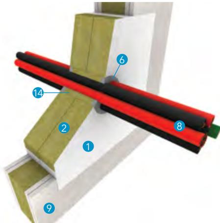
**Detail R - Cable penetration in flexible wall**
