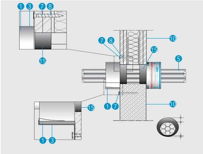
**Detail J - PROMASTOP®-FC MD penetration seal in rigid or flexible wall for single MLC pipe or MLC pipe bundles**
