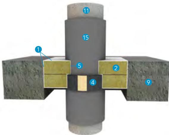
**Detail AE - Non-combustible pipes with combustible local insulation**
