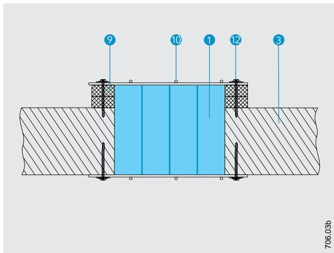
**Detail D - PROMASTOP®-B blank seal in rigid floor**
