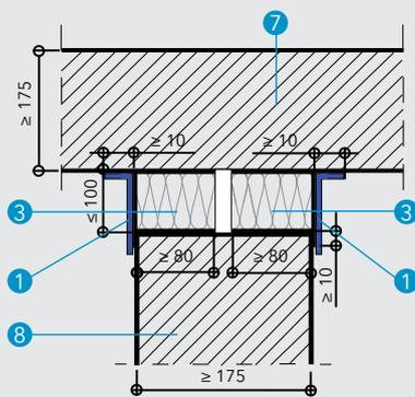
**Detail B - Symmetrical joint filling coated on both sides between wall and steel trapezoid sheet roof**
