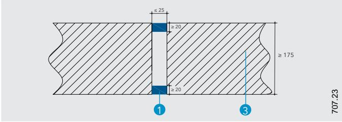
**Detail J - Joint seal without backfilling in floor**
