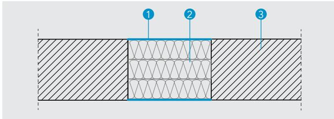
**Detail A - Blank seal made with use of mineral wool and PROMASEAL®-A spray in rigid wall**
