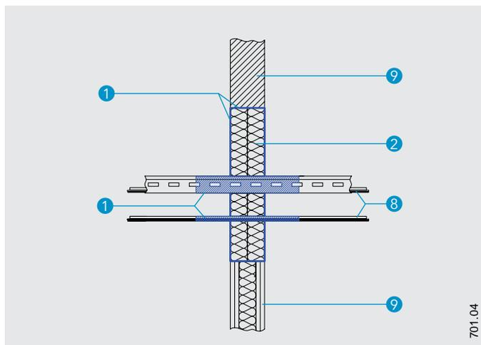
**Detail F - Cable penetration seal in flexible and rigid wall**
