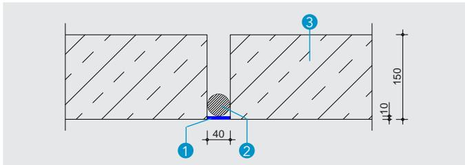
**Detail O** - PP round cord backfilling coated on the exposed side in floor
