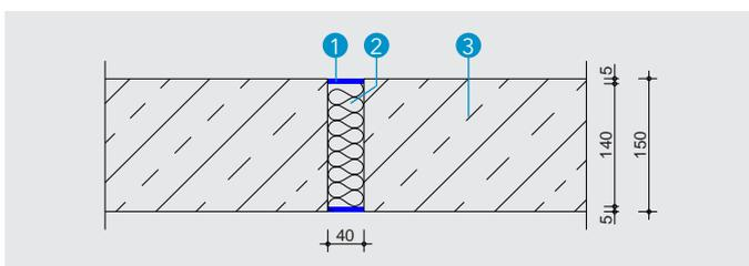
**Detail S** - Mineral wool backfilling coated on both sides in floor
