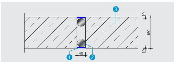
**Detail P** - PP round cord backfillings coated on both sides in floor
