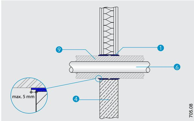
**Detail C - PROMASTOP®-W penetration seal in flexible or rigid wall for pipes with combustible insulation**
