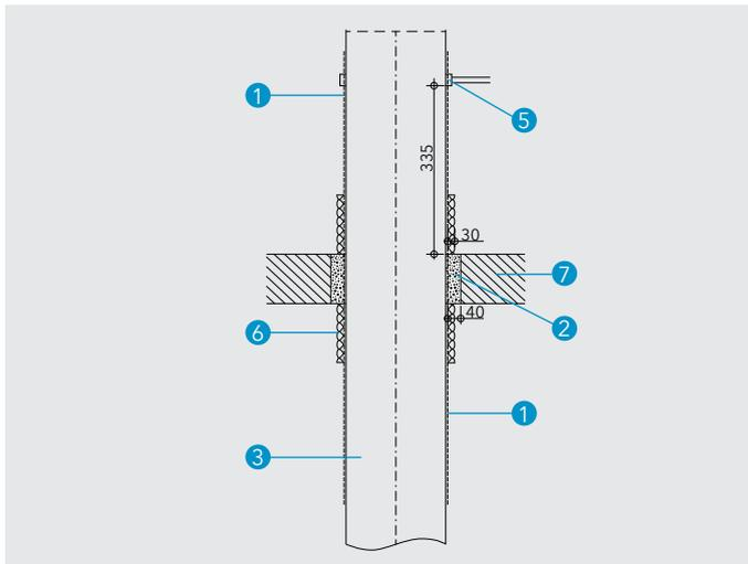
**Detail E - Mortar penetration seal of metal pipes with mineral wool insulation in rigid floor, sealed with use of PROMASEAL®-A spray**
