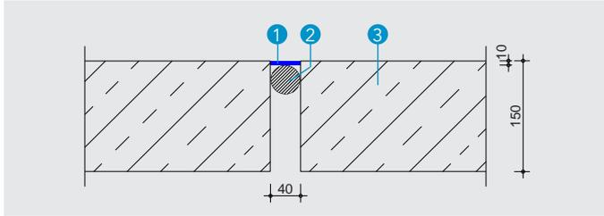
**Detail N** - PP round cord backfilling coated on the unexposed side in floor
