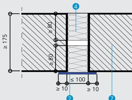
**Detail D - Joint filling coated on the exposed side in floor**
