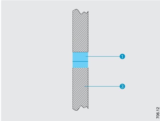
**Detail B - Vertical and horizontal linear joint seal in wall with PROMASTOP®-B**
