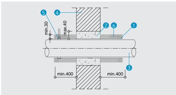
**Detail C - Mortar penetration seal of metal pipes with mineral wool insulation in rigid wall, sealed with use of PROMASEAL®-A spray; the length of the coating on the pipe equal to the length of the insulation**
