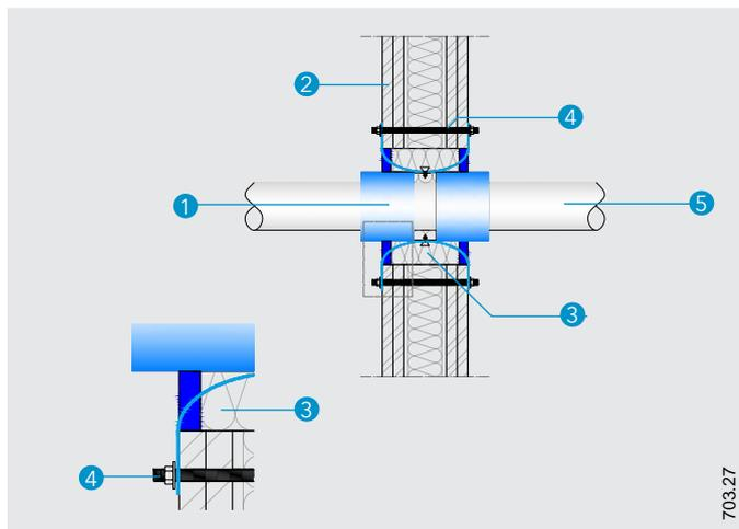
**Detail G - Built-in PROMASTOP®-FC fire stopping collar in flexible wall**
