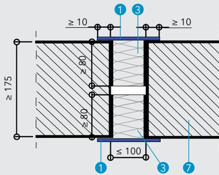
**Detail A - Symmetrical joint filling coated on both sides in floor**
