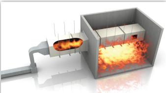
Fire testing for Duct Type B (Exposed to both external and internal fire)
