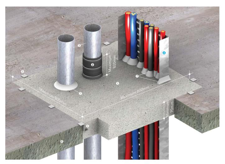
Up to -/240/240 fire resistance in accordance with the requirements of BS 476: Part 20: 1987, BS EN 1366: Part 3: 2009 and/ or AS 1530: Part 4: 2014, depending on applications and types of penetrating elements; insulation time is the measured time to insulation failure on surface of the PROMASEAL® Mortar
