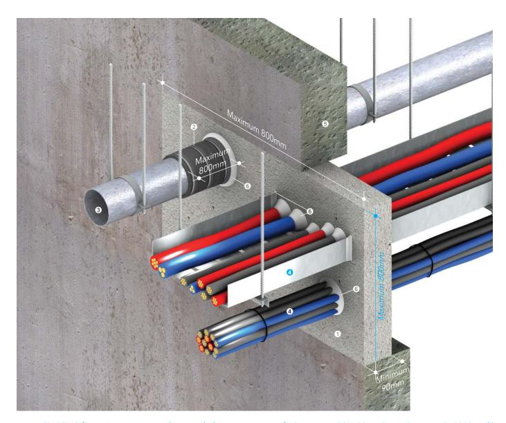
Up to -/240/240 fire resistance in accordance with the requirements of BS 476: Part 20: 1987, BS EN 1366: Part 3: 2009 and/ or AS 1530: Part 4: 2014, depending on applications and types of penetrating elements; insulation time is the measured time to insulation failure on surface of the PROMASEAL® Mortar
