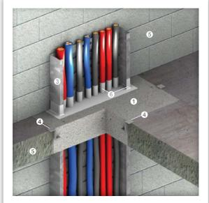
Electrical cables and cable tray passing through concrete/masonry floor with cable tray fixed to shaft wall
