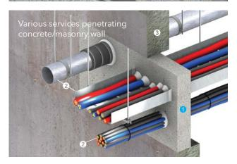
Up to -/240/120 fire resistance in accordance with the requirements of BS 476: Part 20: 1987, BS EN 1366: Part 3: 2009 and/or AS 1530: Part 4: 2014, depending on applications and types of penetrating elements; insulation time is the measured time to insulation failure on surface of the PROMASEAL® Mortar
