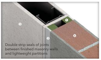
Up to -/240/240 fire resistance in accordance with the requirements of BS 476: Part 20: 1987 and/or AS 1530: Part 4: 2014, depending on applications and types of penetrating elements
