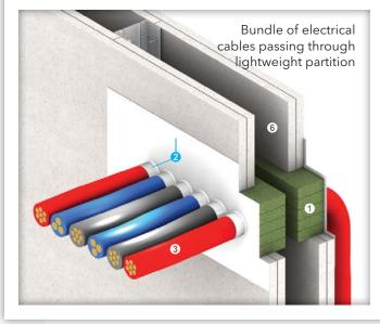
Up to -/240/240 fire resistance in accordance with the requirements of BS 476: Part 20: 1987 and/or AS 1530: Part 4: 2014, depending on applications and types of penetrating elements
