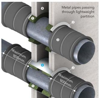
Up to -/240/240 fire resistance in accordance with the requirements of BS 476: Part 20: 1987 and/or AS 1530: Part 4: 2014, depending on applications and types of penetrating elements
