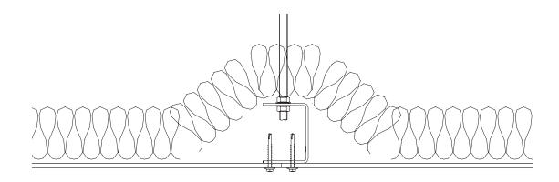
Perimeter channels of ceiling membrane fastened to surrounding construction with M10 or M12 all- steel expanding anchors (or equivalent for alternative types of supporting construction) at 500mm maximum centres.
