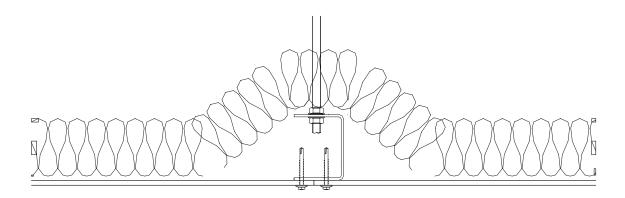
Perimeter channels of ceiling membrane fastened to surrounding construction with M10 or M12 all- steel expanding anchors (or equivalent for alternative types of supporting construction) at 500mm maximum centres.
