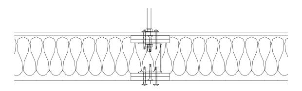
Perimeter channels of ceiling membrane fastened to surrounding construction with M10 or M12 all- steel expanding anchors (or equivalent for alternative types of supporting construction) at 500mm maximum centres.
