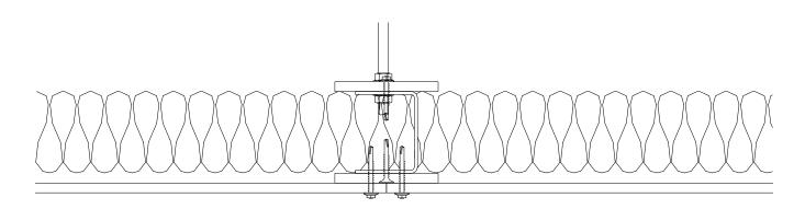
Perimeter channels of ceiling membrane fastened to surrounding construction with M10 or M12 all-steel expanding anchors (or equivalent for alternative types of supporting construction) at 500mm maximum centres.
