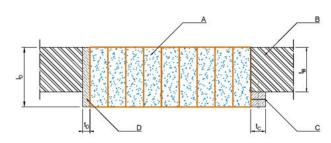
Top view for PROMASTOP®-FB firestop blocks with a length (depth) of 144 mm
