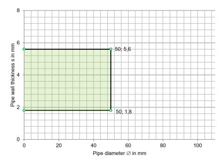
PE-HD pipes according to EN 1519-1 and DIN 8074 / DIN 8075 with diameters and wall thicknesses as defined above. For interpolation between pipe diameters and wall thicknesses see diagram below.
