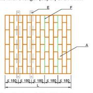
Top view for PROMASTOP®-FB firestop blocks with a length (depth) of 200 mm
