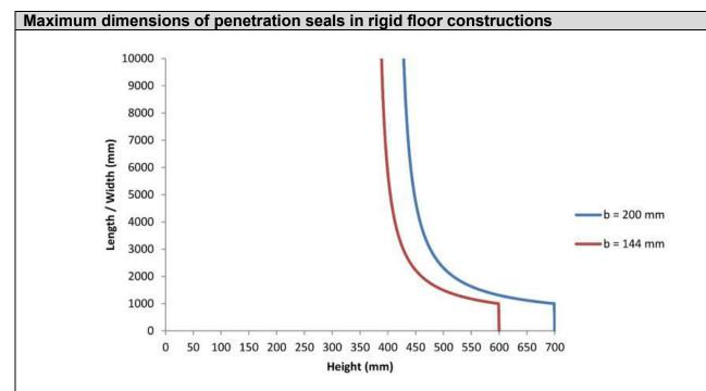
The maximum length (width) of the seal in rigid floors has to be calculated as follows:
