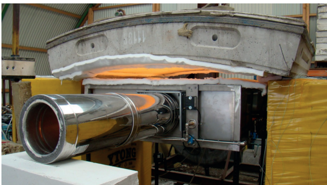
Efectis full mobile furnace with segment
