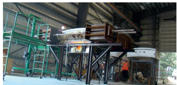
Port of Miami Tunnel Efectis mobile test setup
