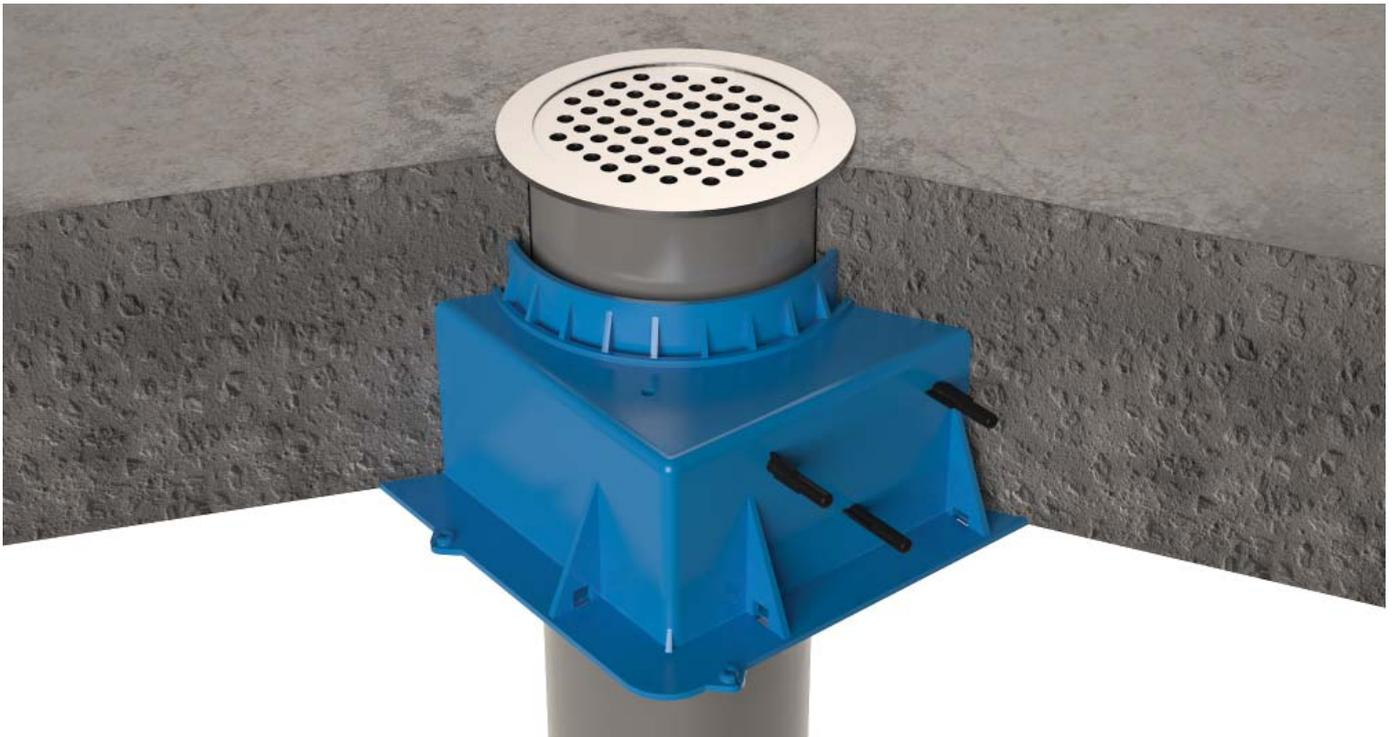
Floor waste collars help prevent the passage of fire and smoke through openings in compartment floors in the event of a fire. For installation of collars on permanent form work and in thin floor slabs (<150mm) please consult Promat. These collars are available in various models and their applications depend on the certification required for the building.
